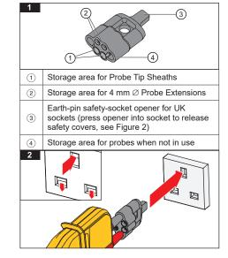
Figure 3 illustrates how to store and retrieve the tip accessories from the cap.
