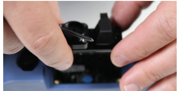
The power meter and VFL piece are offered as an easy-to-install option that's as simple as removing four screws.
