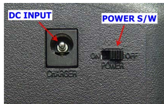
<Figure 3. Power supply at the back>
