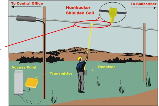
To calibrate the Receiver, search about a 3' [1m] section for Peak Tone
