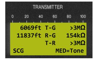
R-G Ohms indicates the unbalance **is not** a one sided open. The 154k Ohms is an AC Ohms indication and will not be the same as your DC Ohmmeter until the pairs you are crossed with are identified and grounded.
