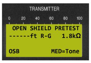
If the R-G length is dashed out you cannot get an estimated distance to the fault, continue toning the fault.
