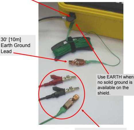
Clips of 3 wire test lead
