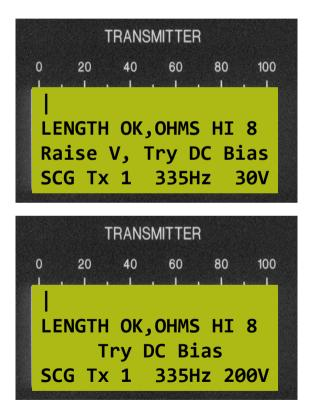
When a high resistance fault will not produce adequate tone for tracing, the DC BIAS will dislodge any insulating oxide layer present to bring faults **up to 1M Ohm** down into the Locatable Fault Range, especially in PIC cable.
