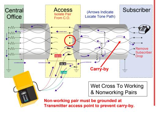
In a Wet PULP Fault many adjacent pairs are crossed with the toned pair. To reduce carry-by, bunch several adjacent pairs involved in the wet and ground to the Transmitter Green ground lead.
