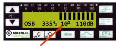
0° to 45° means you are approaching a Shield-to-Earth fault
