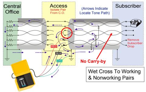
The crossed non-working pair has been grounded. In Wet PULP cables multiple crossed pairs should be grounded.
