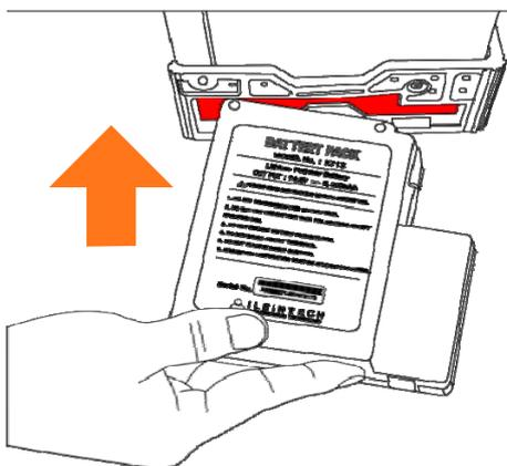
Insert the battery into the battery groove until it clicks.
