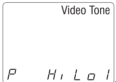
Figure 12. Video Cable Test with Pin Selected
