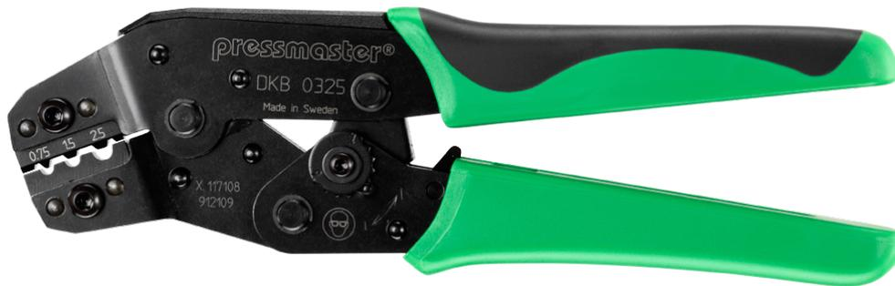
DKB-0325 is a crimping tool for non insulated connectors, 0.35-2.5 mm<sup>2</sup>/AWG 22-14, Indent-Crimp.
