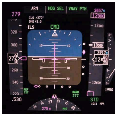
EFIS with 2 1/2 Dot ILS Deviation Figure 4
