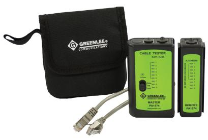
The PA1574 from Greenlee Communications tests the continuity of 8-way (RJ45) data and network and 6-way (RJ11) telephone patch cords and installed cable runs. It maps the cable, line by line and identifies good connections, opens, shorts and crosses. Includes patch cords, 9V battery and carrying pouch.
